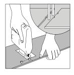
Holes for pipes: measure the diameter of the pipe and drill a hole that is 20mm (7/8") larger. Saw off a piece as shown in the figure and lay the board in place on the floor. Then lay the sawed-off piece in place.
