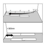
(5) Start the second row with the leftover cut part of the last plank of the previous row. This small plank should measure at least 30cm (12"). Otherwise, use another plank that should be cut in two. At any case, the short sides cut are distant from at least 30cm (12").
