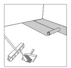
① After thoroughly cleaning the subfloor, you should install a foam underlay (unless your product has a pre-attached pad). Run the foam underlay in the same direction as the flooring planks. The underlay should be butted side-by-side with no overlap. Tape seams together. If you are installing over a concrete suboor, a 6-mil poly (plastic sheeting) is to be installed under the foam underlay. (Many foam underlays already have this plastic sheeting pre-attached).
